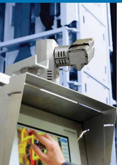
The Bentec COLOR CAMERA SYSTEM allows users to monitor the whole drilling rig from one central point and view places with limited visibility in a safe and reliable way.
